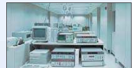
Temperature- and humidity-controlled calibration room
